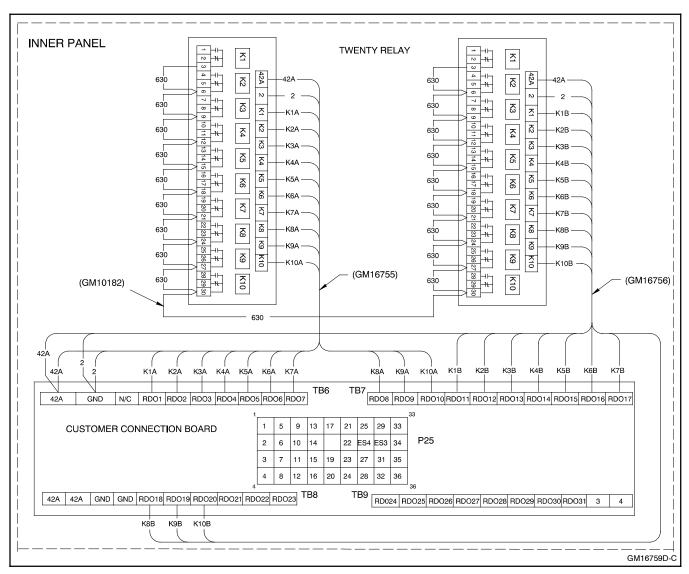
Figure 6-35 Twenty-Relay Dry Contact Relay Kit Connections
